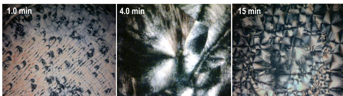
Figure 1. Polarized optical microscopy of PCL-PEG 50%/50% networks. Isothermal recrystallization at room temperature (material was first taken to the melt and then quenched to room temperature).
